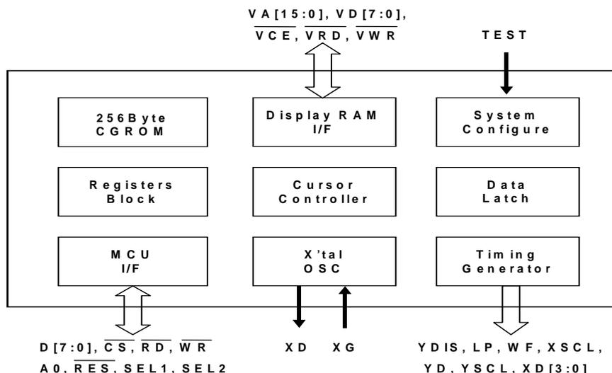
Figure 3-1: Block Diagram
