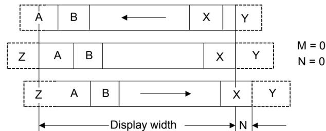
M/N is the number of bits(dots) that parameter 1 (P1) is incremented/decremented by.
