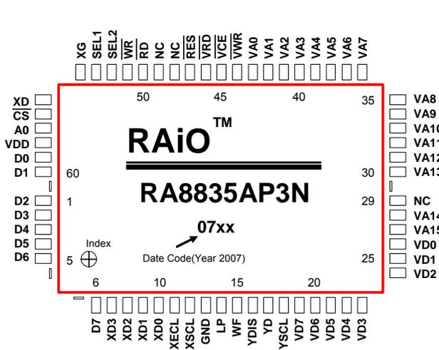
Figure 4-1: RA8835AP3N(QFP-60 Pin)
